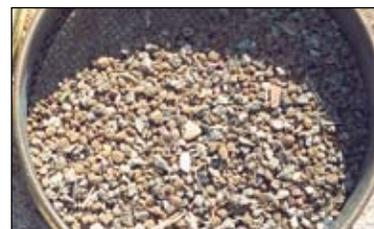
Figure 4. Separation of particles larger than 2 mm but smaller than 5 mm.
