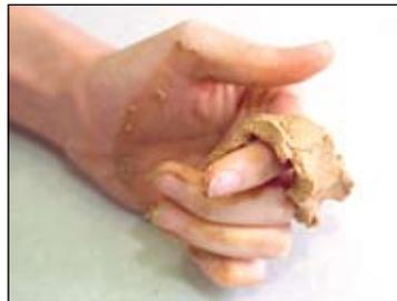
Figure A4. Class III soil (Silt loam—16 percent clay, 19 percent sand, 65 percent silt).
