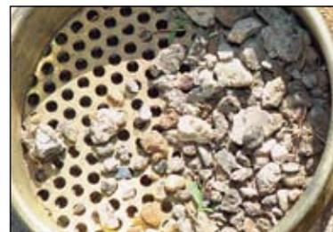
Figure 5. Gravel particles larger than 5 mm from soil sample.
