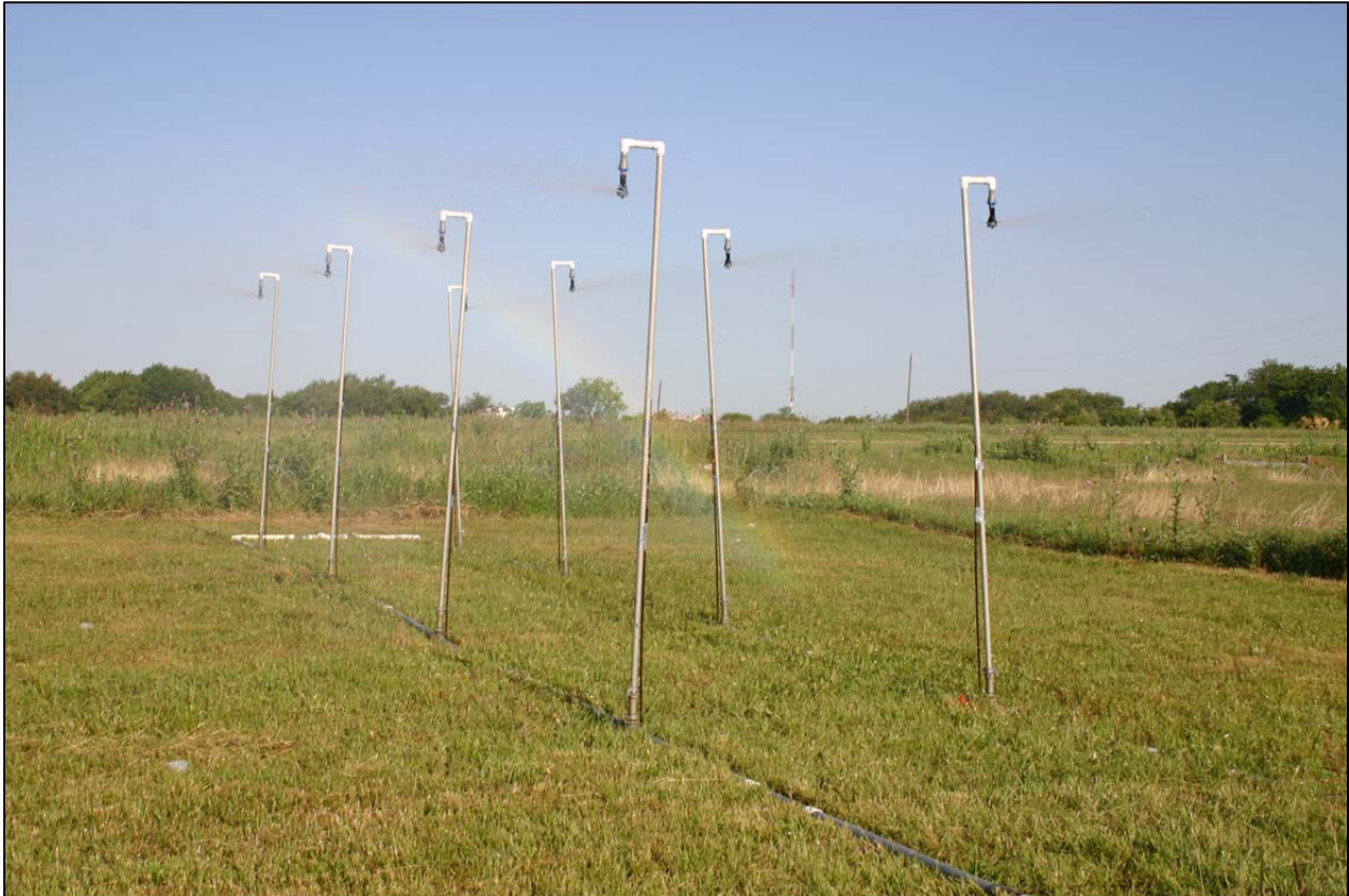
Runoff generation on grassland plots using simulated rainfall. Whitish objects in plot area are plastic rain gauges used to monitor rainfall amounts.
